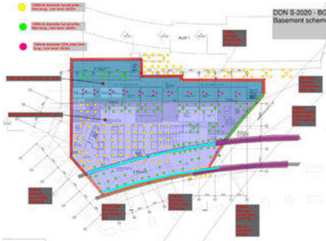
Fig 6.2.69: Interface between Basement and Retaining Secant RC Walls
