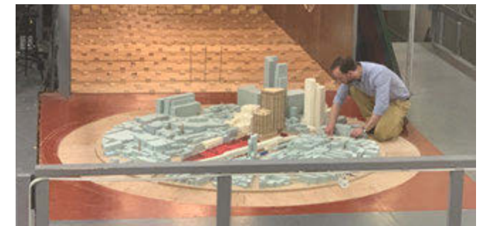
Fig 6.2.46: Wind tunnel testing for Plot 2 and masterplan
